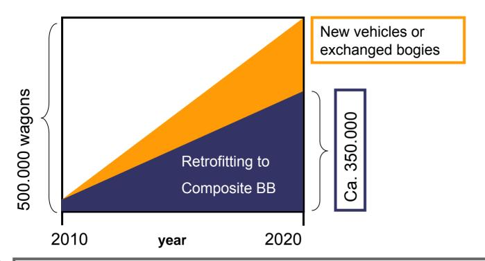
To meet acceptable noise emission values till 2020, most of the freight wagons have to be equipped with composite brake blocks. 1/3 will be new vehicles, 2/3 have to be retrofitted.
