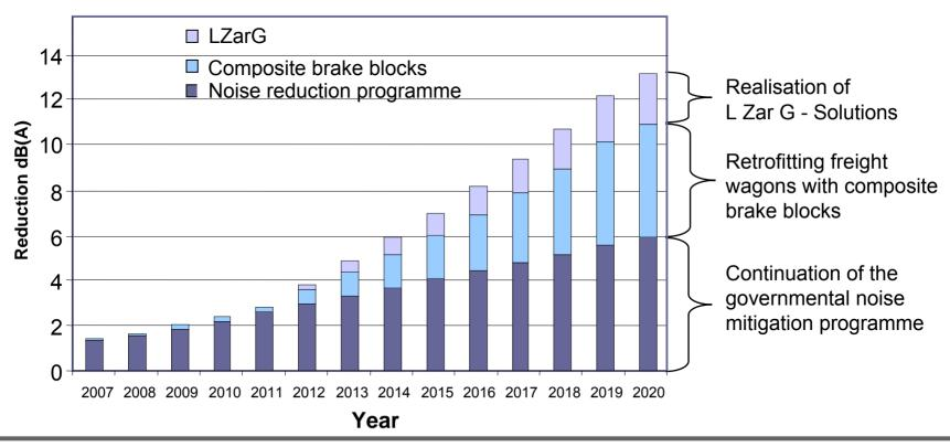
Reaching the noise mitigation target of DB depends mainly on the successfull introduction of composite brake blocks. LäGiV shall assure that from 2013 onward LL- blocks will be availabe, which offer safe operation and cost effective retrofitting of freight wagons. Retrofitting with K – blocks would triple the costs.
